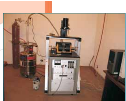
Magnetometru Micromag AGM/VSM model 2900/3900
