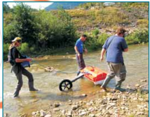
Georadar model SIR-3000 Ground penetrating radar SIR-3000
