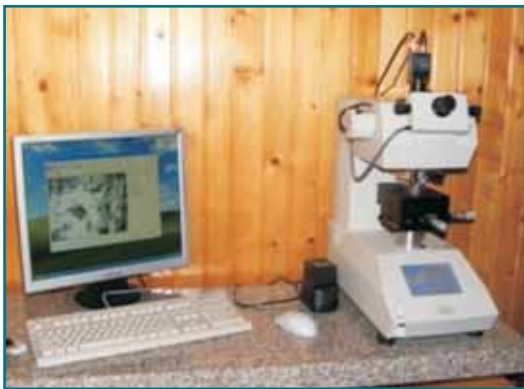
Martens Hardness tester with gradually applied load (Laboratory of testing and materials characterization)
