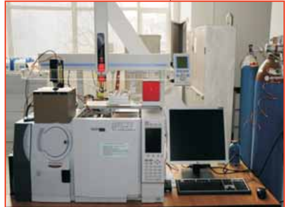
Analizor GC-MS Gas cromatograph mass spectrometer analyzer
