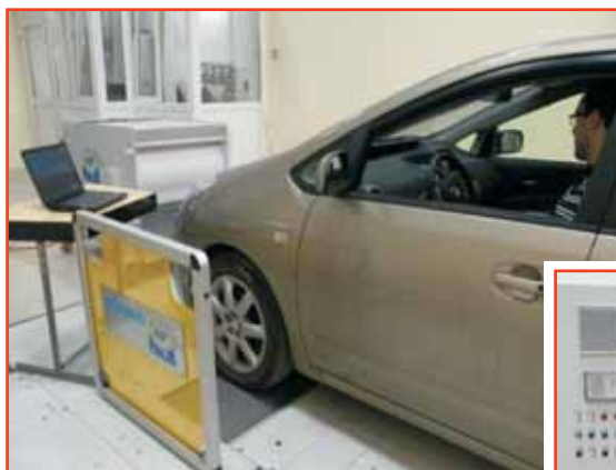
Stand dinamometric cu rulouri tip MAHA 2 WD ECMD 48L/LD
