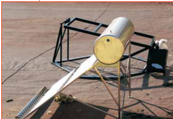
Colector solar termic Thermal solar collector
