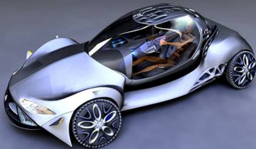
Body parts made out of Loprefin
