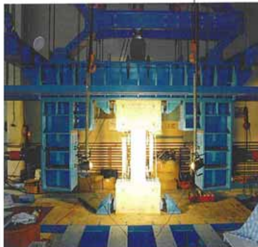
Fig. 1 - Reactive frame mounted in the Structural Testing Laboratory
