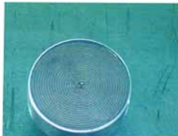
Very wide band Archimede's spiral antenna for warning stations
