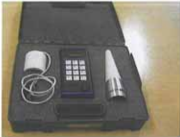
Magnetic programmer for proximity and high explosive fuses
