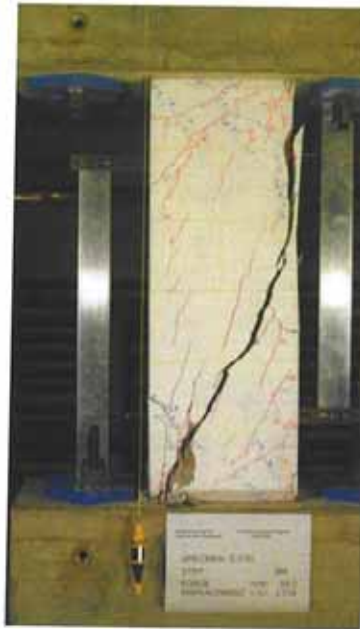
Figure 4. Reinforced concrete pillar tested in the laboratory
